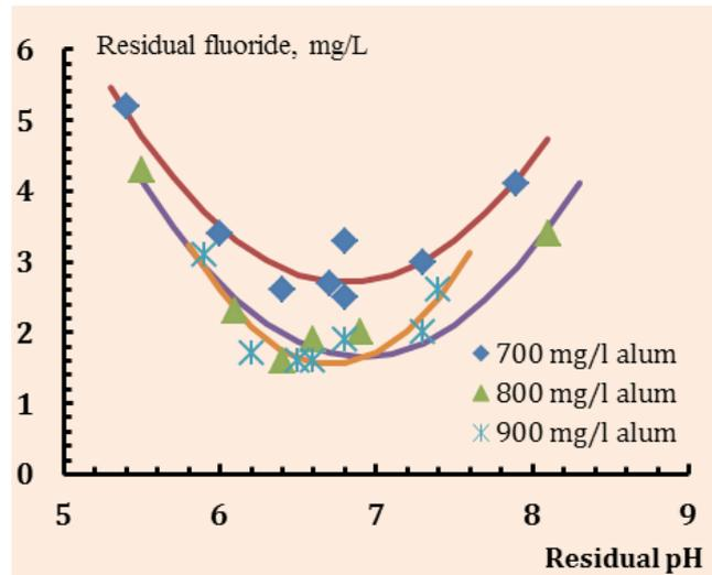
**Figure 6.** Fluoride removal in batch by adding alum and lime to water containing 12.2 mgF/L.
