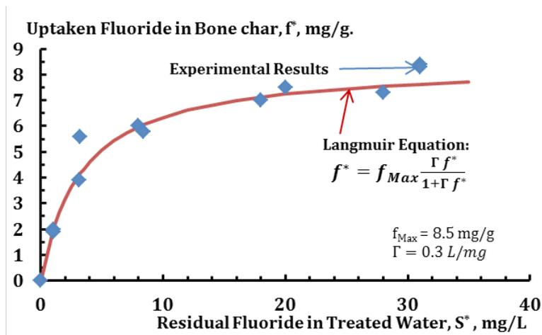
Figure 11. Match of fluoride removal experimentally and theoretically using bone char and the Langmuir sorption model.
