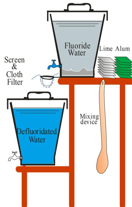
**Figure 7.** The Nalgonda technique setup as developed for use households.
