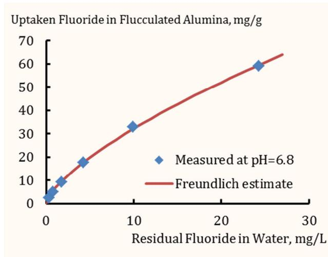
**Figure 4.** Match of fluoride removal experimentally and theoretically using alum and Freundlich model and where pH is kept at 6.8
