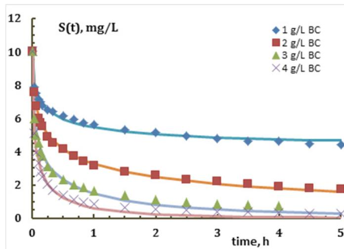
**Figure 12.** Fluoride uptake on batch chemostate where pH is kept at 7.0. The dots are discrete experimental data while the corresponding curve is given by the kinetic model.
