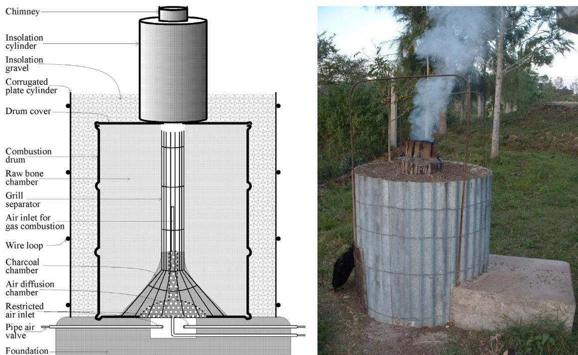
**Figure 13.** The charcoal kiln for preparation sorption media, a significant development made by the DTP toward appropriate defluoridation of water in developing countries.
