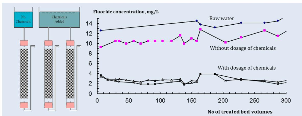
**Figure 8.** Illustration of the contact precipitation as run in columns. Left triple column setup filled with saturated bonechar and run with and without addition of calcium and phosphate from [23].
